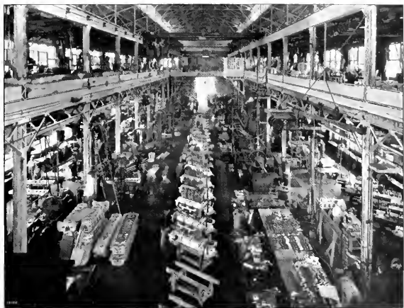
View in the main bay of the erecting shop of the Consolidated Shipbuilding Corporation, showing large number of Speedway engines in process of erection on the floor.
